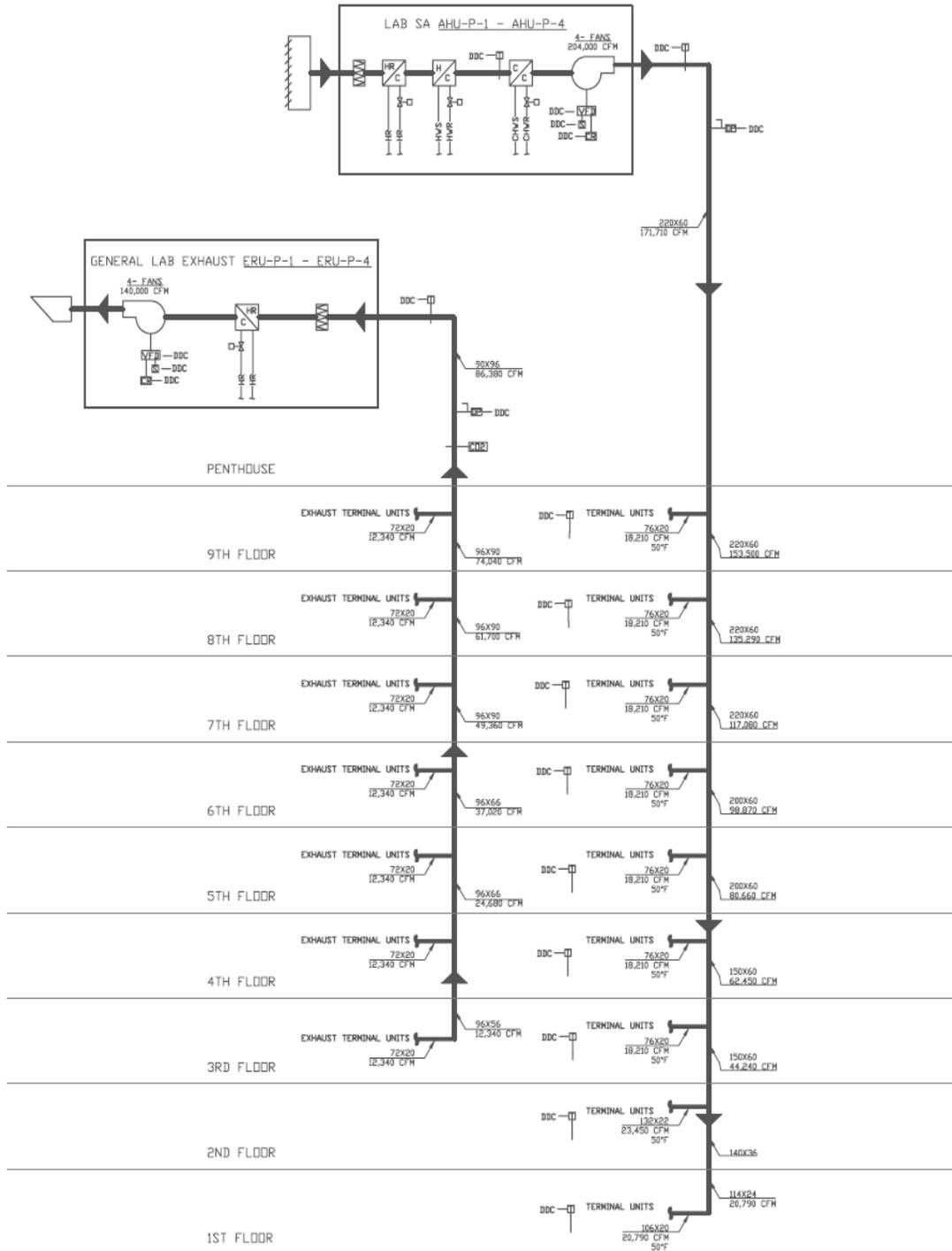
S.5 LAB SUPPLY, GENERAL LAB EXHAUST SCHEMATIC
